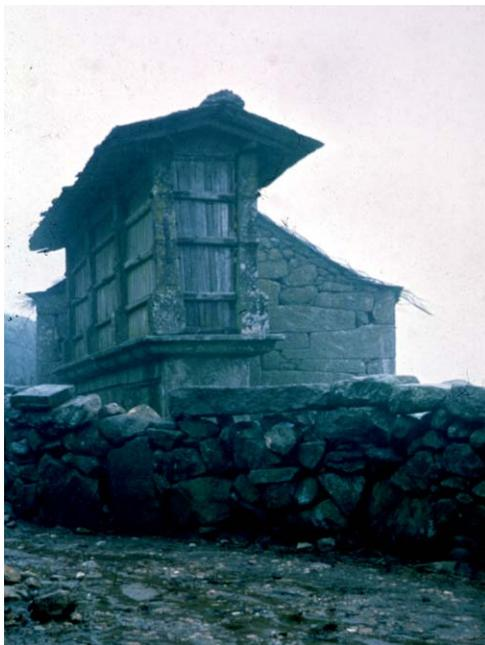
Gerês. Corn Silo. Ventilated structure used to store corn cobs. These structures of rural architecture have a very expressive presence.
